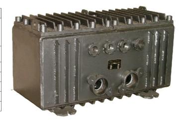
The flameproof box of SFIS inverters and controllers, as a flameproof enclosure, is made in the form of a cuboid with dimensions of  $\sim$  460 mm (height) x  $\sim$  445 mm (depth) x 920 mm (width).
