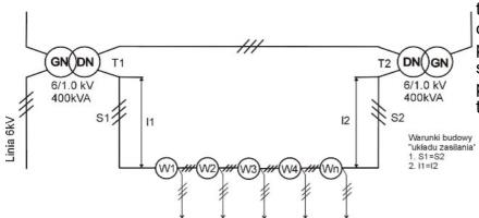
to supply mining longwall complexes of increasing power. The power supply system allows full use of the power of two IT3Sb or IT3Sd transformer stations.
