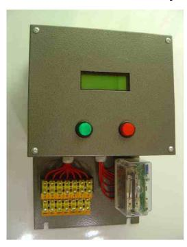
The RPW-1 type relay is built based on the microprocessor technique.
