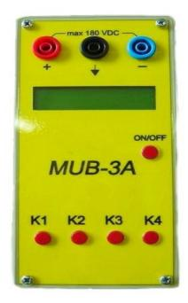
The MUB-3A battery leakage meter may only be used in rooms with no methane explosion hazard - grade "a" and classified as class "A" of coal dust explosion hazard.
