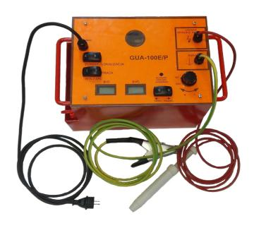
In the shock-acoustic generator with the GUA-100E / P measurement, the method of using the optical-acoustic effects accompanying the impulse breakdown of insulation with the test voltage (adjustable up to 20kV) at the point of damage to the conductor of the tested cable or sheathing conductor was used for the location of damage to cables or tire conductors. The shock-acoustic generator with the GUA-100E / P measurement can work in the measurement and location modes.
